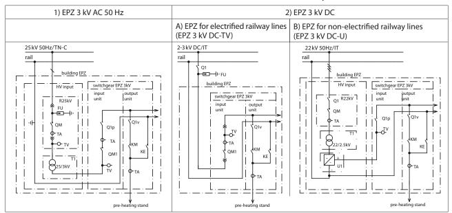
If no traction system is available as a source of power (along non-electrified railway lines), direct power system EPZs may also connect to the 22 kV AC/IT distribution three-phase power system (as well as to another high-voltage 6, 10, 35 kV AC/IT power systems).
